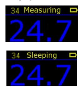
Detect the PM2.5 concentration every 5 minutes. Collect the surrounding air in 60 seconds, then display the result which is the mean. The model is suitable for long time detection of particles in the environment ,and the monitor can work more than 30 hours under this model.
